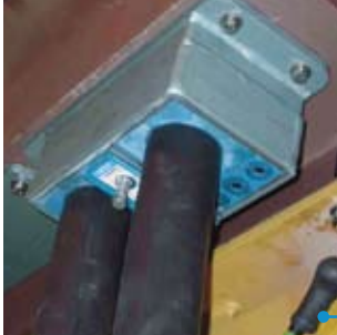
Roxtec S 4x1 in the floor of the driver's cabin of a giant mining dump truck. Used for mechanical anchorage of cables and reduction of vibration.
